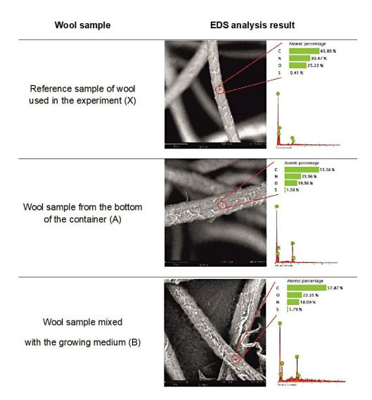
Figure 4. SEM microphotographs along with the results of EDS qualitative analysis
